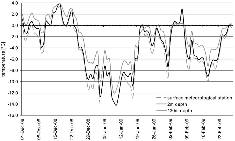
Fig. 5. Minimal air temperatures in the cold period.
