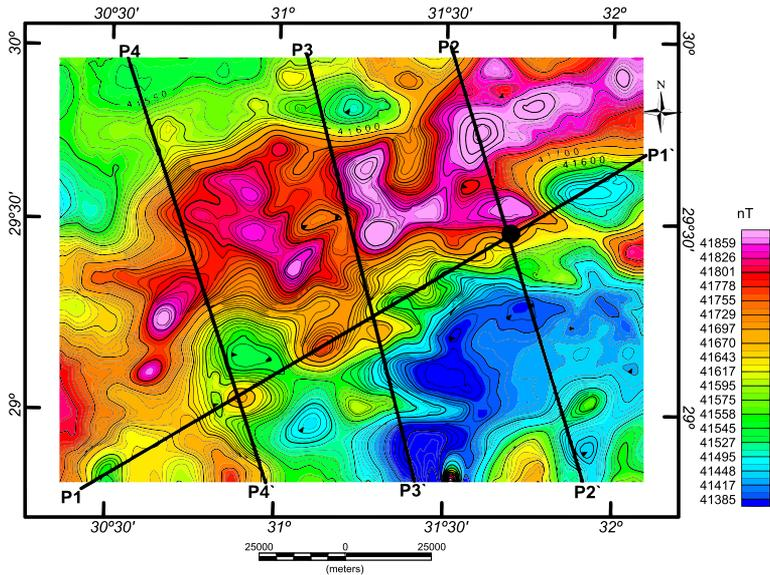
Fig. 4b. RTP aeromagnetic map of the studied area.
