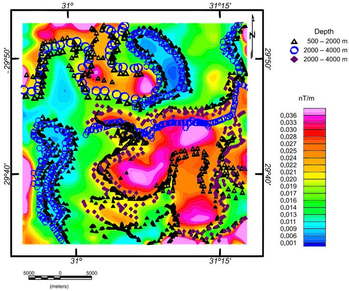
Fig. 7a. The Euler convolution for magnetic map of the studied area.
