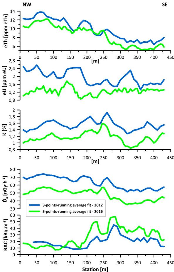
Fig. 5. The courses of repeated radiometric quantities measured in years 2012 and 2016 along the same profile.
