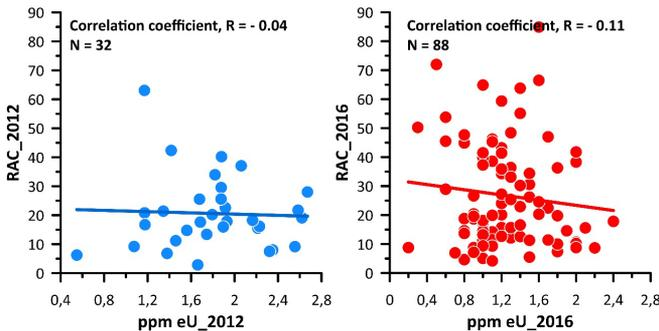
Fig. 7. Linear correlation (R) between uranium and radon in soil in 2012 and 2016 years.
