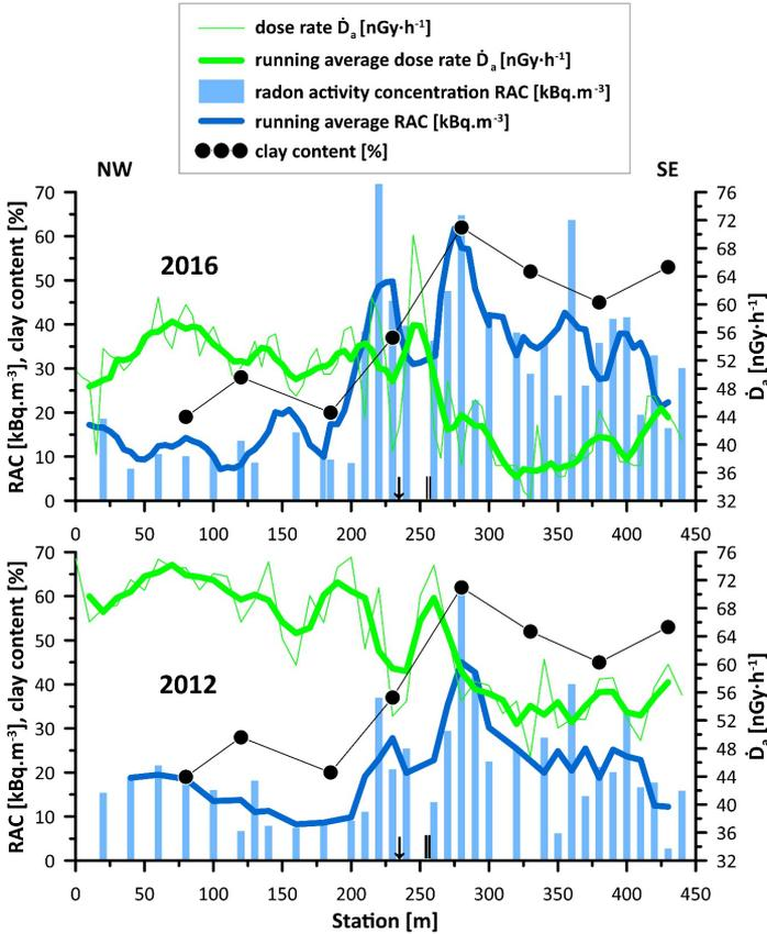
Fig. 3. The results of ground gamma-ray spectrometry and soil radon emanometry measured along the same line in 2012 and 2016 years (explanations: ↓ – map fault position, || – concrete road position).
