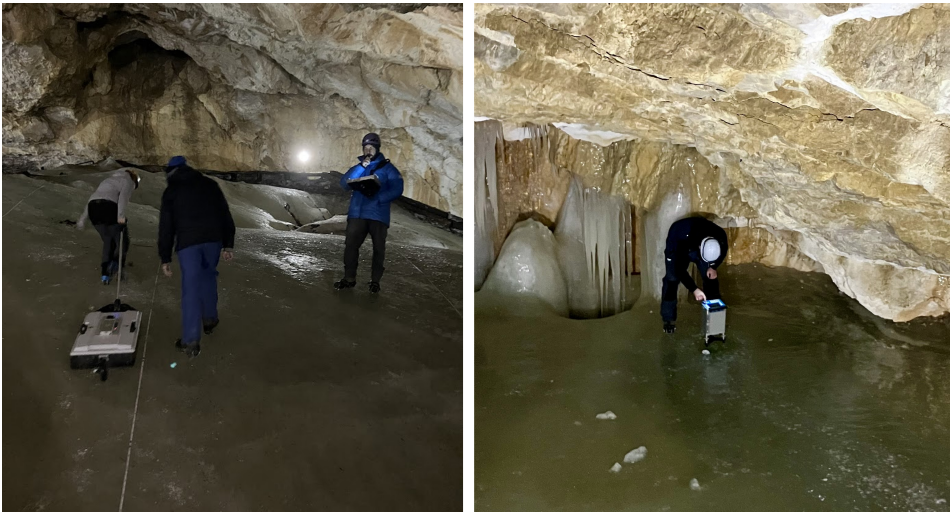
Fig. 1. Geophysical data acquisition in the Dobšiná Ice Cave (left: georadar measurements, right: gravimetrical measurements).
