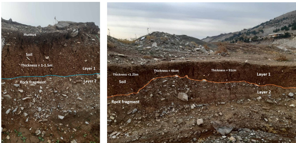
Fig. 2. Photo image shows the layer thickness and types of layers.
