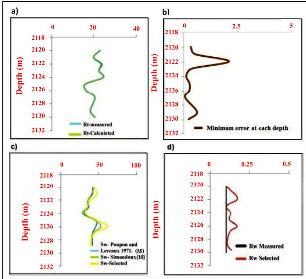
Fig. 5. (a) The measured and the calculated  $R_t$  curves; (b) Minimum error between the measured and the calculated  $R_t$ ; (c) the calculated  $S_w$  from different equations and the selected  $S_w$  from the proposed technique; (d)  $R_w$  measured and the selected  $R_w$  from the proposed technique.
