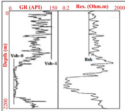
Fig. 1. Determining  $R_{sh}$  using GR and Resistivity log.
