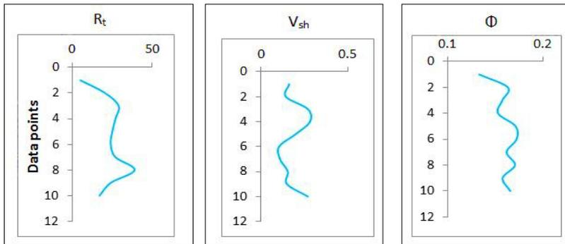
Fig. 3. Synthetic example for  $R_t$  and  $V_{sh}$  which is used to create  $\phi$ .
