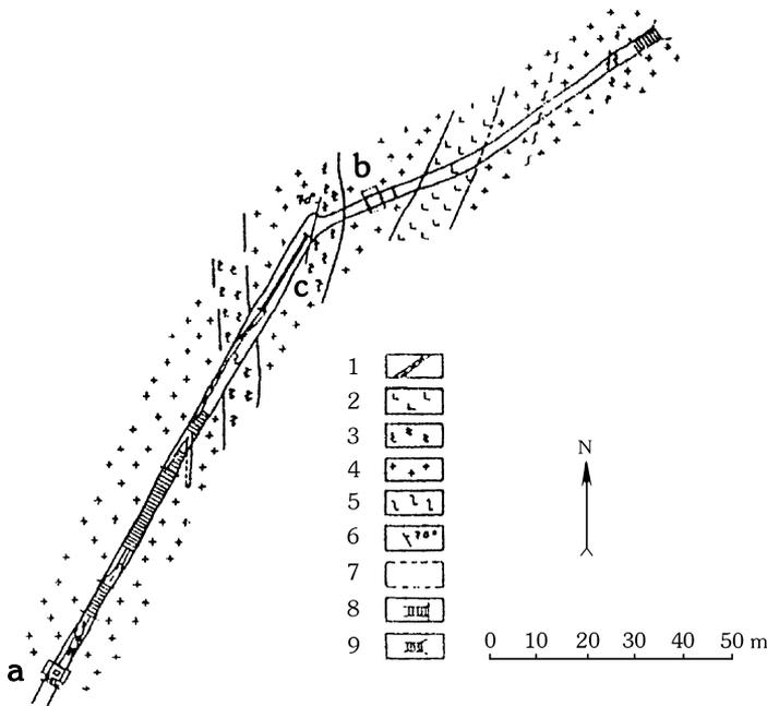
Fig. 1. Tidal station in the Vyhne. Geologic and tectonic situation in the Anton Paduánsky gallery: 1-granite zone with mylonites and quartz; 2-Dacite (Neogene); 3-ancient zone in granite; 4-granite (Vyhne ancient granite - Palaeozoic); 5-fault; 6-fault with its slope; 7-location of instruments (a-tiltmeter chamber, b-recording instrument chamber, c-extensometer); 8-walled-up areas; 9-entrance to gallery.
