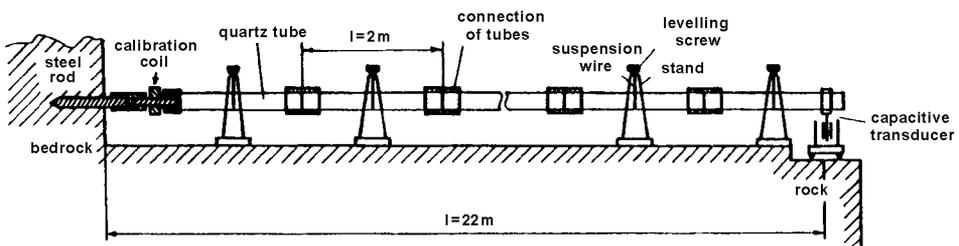
Fig. 2. The fundamental design of the rod extensometer.
