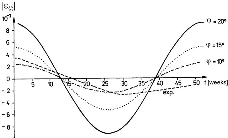
Fig. 5. The time variation of the computed elastic deformations for the slope inclined at angle  $\varphi = 10^\circ$  (dot-dashed curve),  $\varphi = 15^\circ$  (dotted curve),  $\varphi = 20^\circ$  (solid curve) and the slow deformations observed at the Vyhne station (dashed curve).
