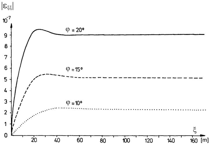
Fig. 6. The dependance of the amplitudes  $|\varepsilon_{\xi\xi}|$  of the calculated thermo-elastic deformations on the distance from the free boundary for the slopes inclined at angles  $\varphi = 10^\circ$  (dotted curve),  $\varphi = 15^\circ$  (dashed curve),  $\varphi = 20^\circ$  (solid curve).
