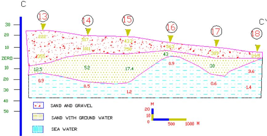
Fig. 9. Goelectric cross-section C-C'.
