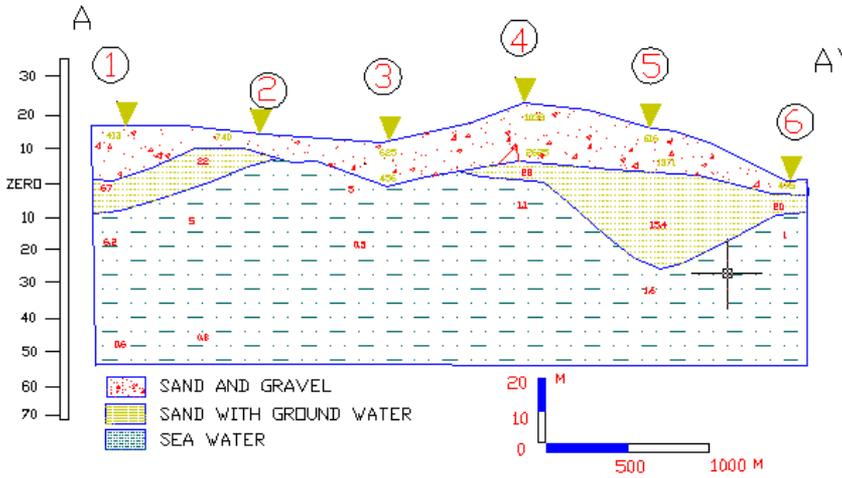
Fig. 7. Goelectric cross-section A-A'.
