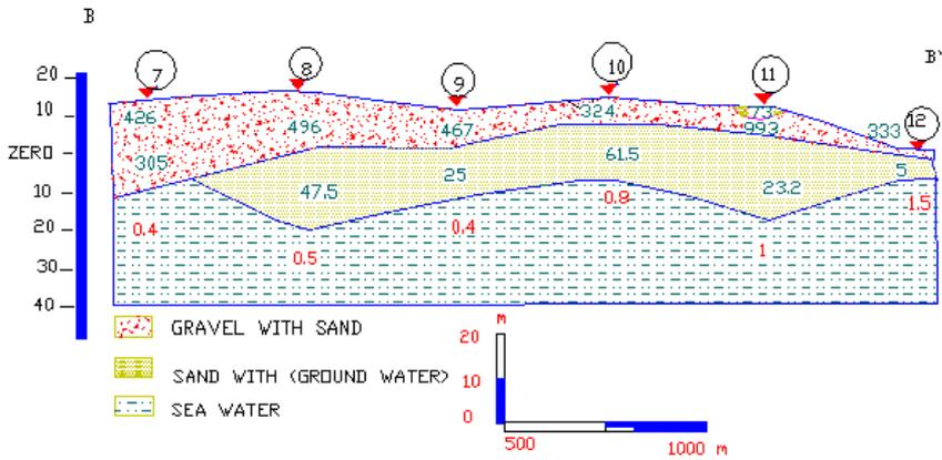
Fig. 8. Goelectric cross-section B-B'.
