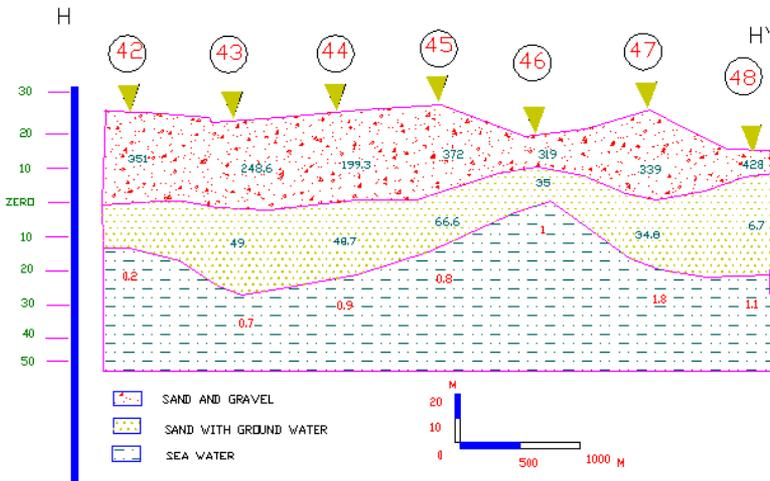
Fig. 14. Geoelectric cross-section H-H'.
