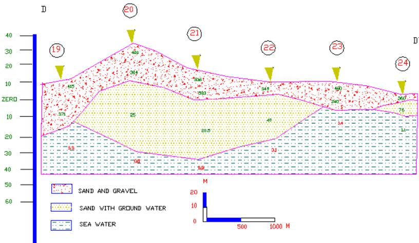
Fig. 10. Goelectric cross-section D-D'.
