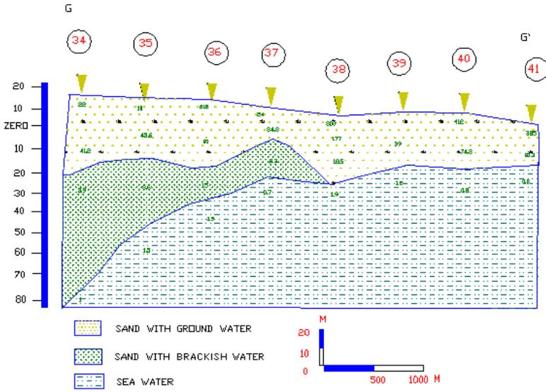
Fig. 13. Geoelectric cross-section G-G'.
