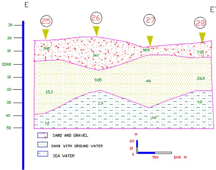
Fig. 11. Geoelectric cross-section E-E'.
