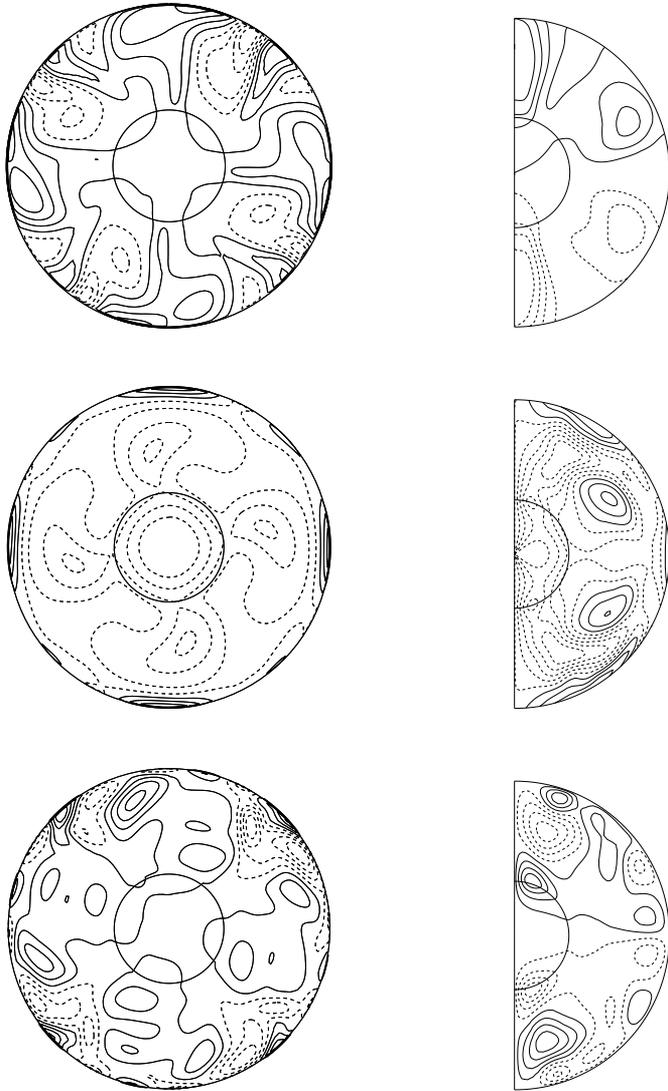
Fig. 3. Magnetic field components ( $B_r, B_\theta, B_\varphi$ ) (from top to bottom); equatorial (left column) and axi-symmetrical meridional (right column) sections, for  $E = 10^{-4}$  and  $q = 2$ .
