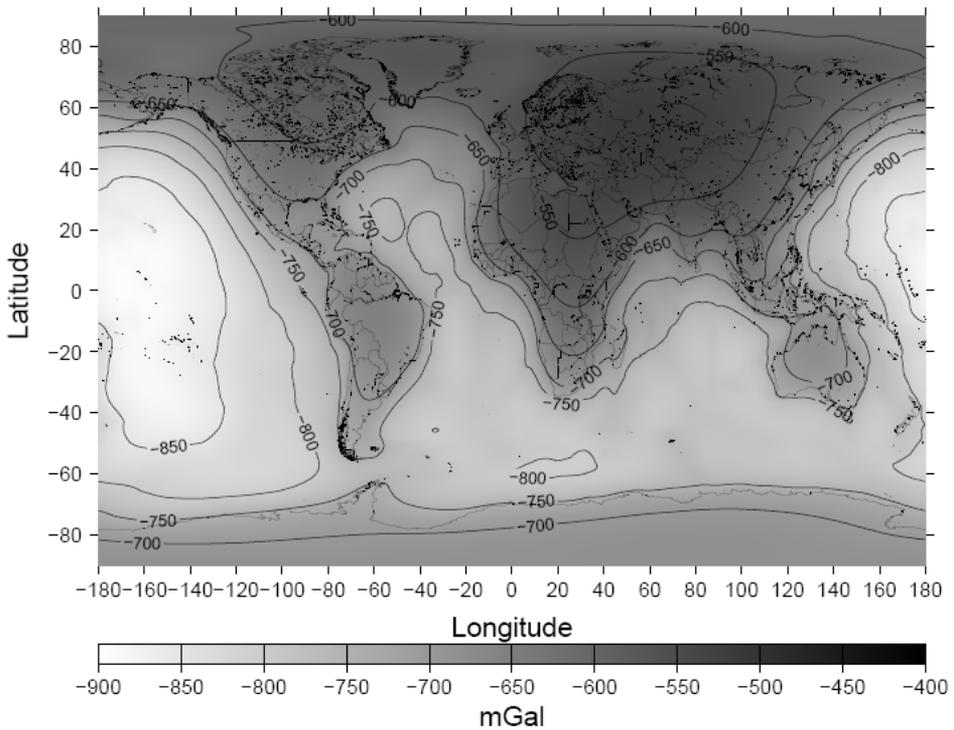
Fig. 2. The global secondary indirect bathymetric effect at the Earth's surface computed with the spectral resolution complete to degree 180 of spherical bathymetric functions. The mean value of the ocean density contrast  $-1640$  kg/m<sup>3</sup> was adopted.
