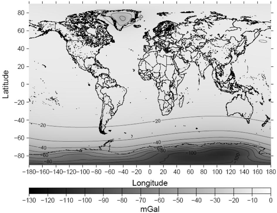
Fig. 3. The global secondary indirect ice density contrast effect at the Earth’s surface computed with the spectral resolution complete to degree 90 of spherical ice thickness functions. The mean value of the ice density contrast  $-1757 \text{ kg/m}^3$  was adopted.
