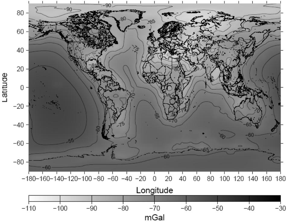
Fig. 4. The global secondary indirect sediment density contrast effect at the Earth's surface computed with the  $1 \times 1$  arc-deg spatial resolution.
