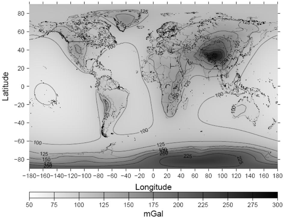
Fig. 1. The global secondary indirect topographic effect at the Earth’s surface computed with the spectral resolution complete to degree 180 of spherical height functions. The mean crustal topographical density  $2670 \text{ kg/m}^3$  was adopted.
