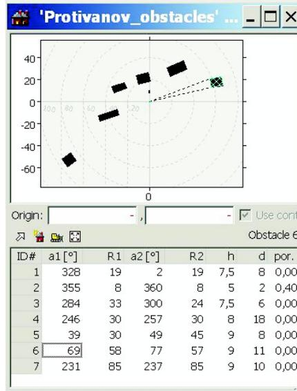
Fig. 6. Obstacles near the Protivanov CHMI meteorological station as viewed in WAsP.
