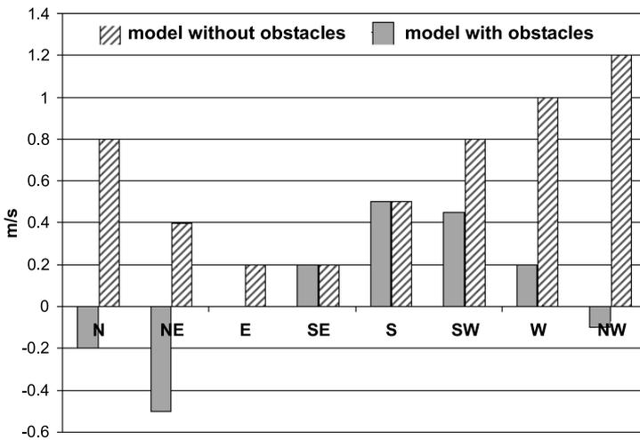
Fig. 7. Sector-wise differences between the measured and extrapolated values of mean wind speed. Extrapolation performed by WAsP from station 2 to station 1 according to Table 1.
