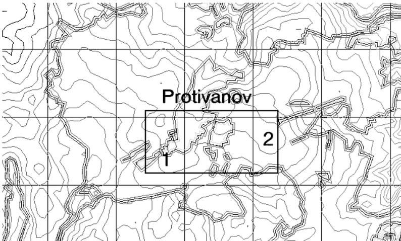
Fig. 5. Orography and roughness layers in the area approx.  $6 \times 3.5 \text{ km}^2$  near Protivanov viewed in WAsP. The smaller rectangle covers an area of  $2 \times 0.9 \text{ km}^2$  for detailed calculation with a 10 m resolution in the horizontal. Numbers 1 and 2 correspond to the sites with wind measurements according to Table 1 (site 3 is situated outside of the map area).
