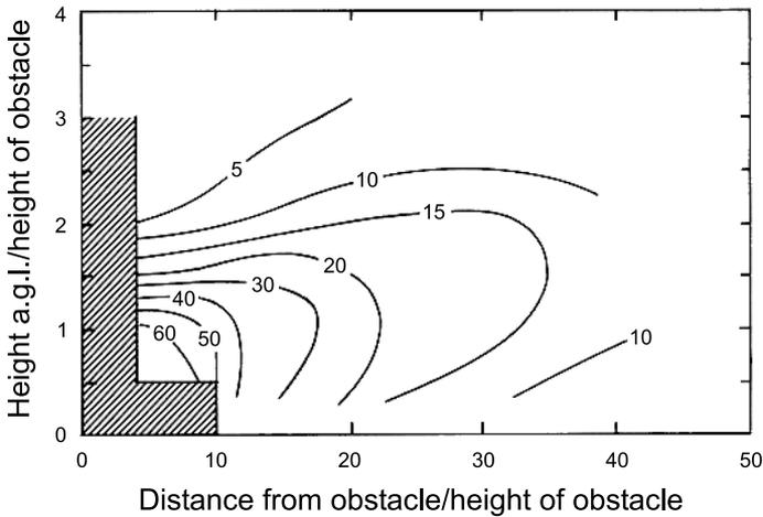
Fig. 1. Reduction of wind speed (%) due to shelter from an infinitely long two-dimensional obstacle of zero porosity. Based on the expressions given by *Perera (1981)*.
