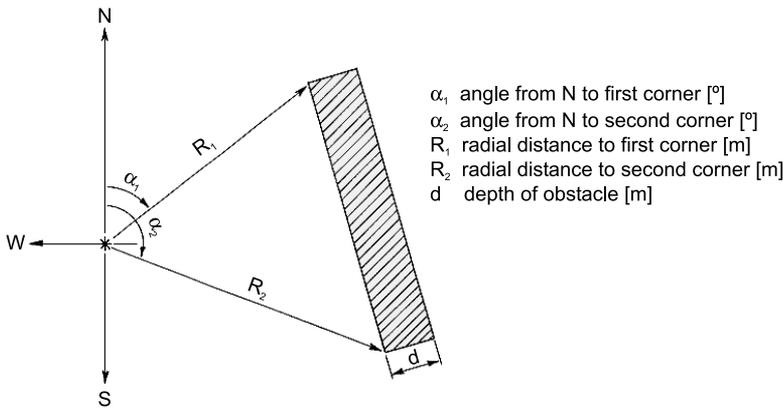
Fig. 2. Quantities that specify a single obstacle and that must be input into WAsP. Obstacles are specified as rectangular boxes relative to the site: by two angles, two radii, their height, depth and porosity.
