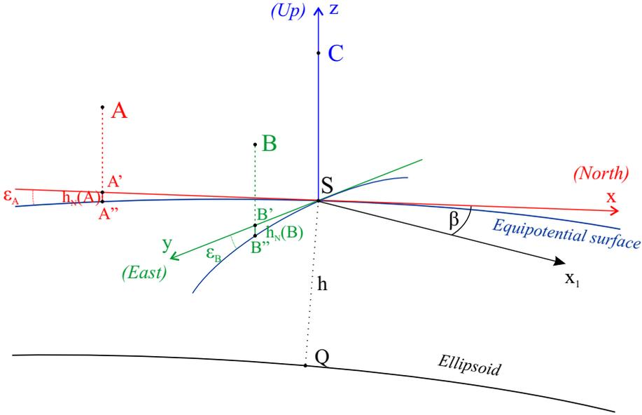
Fig. 1. The geometry of the local gravimetric network, showing the main concepts and the quantities involved in the computations.
