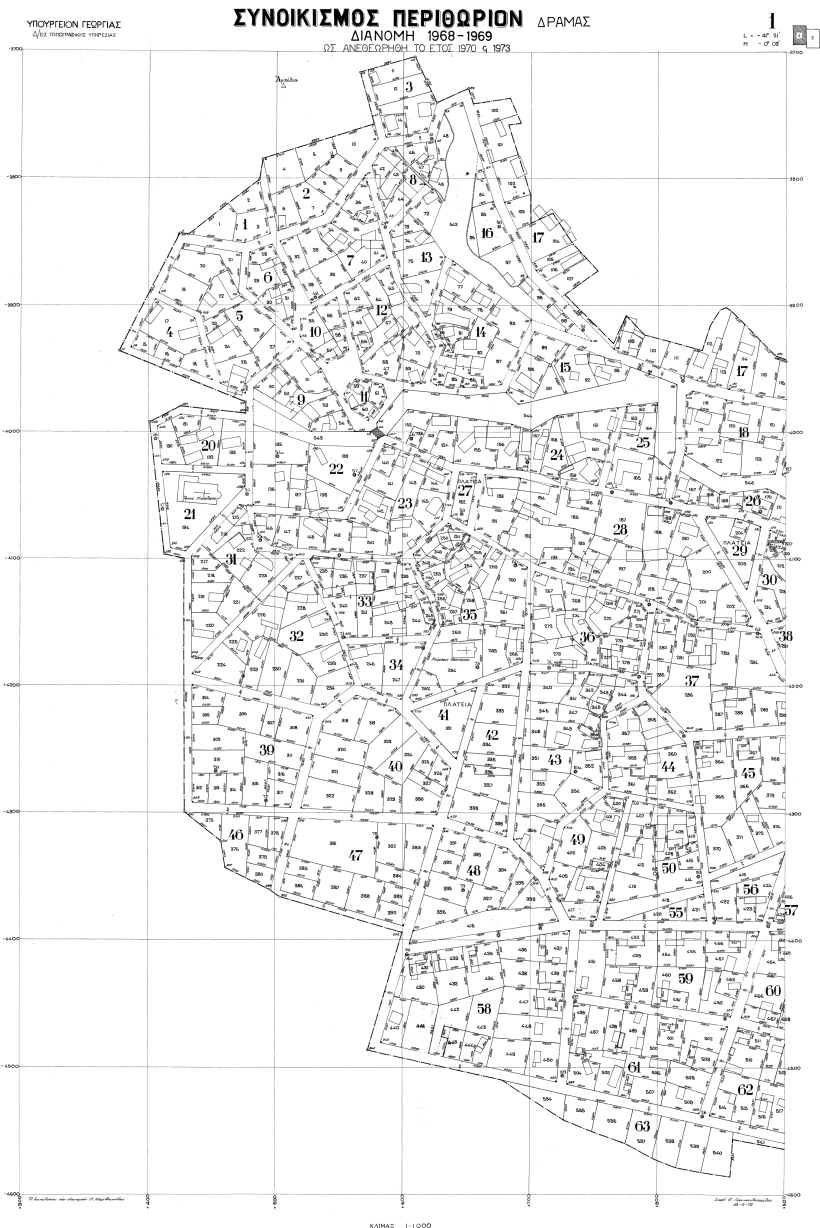
Fig. 2. The associated map sheet of Perithorion with respect to the “old Bessel” (scale 1:1000, credits to the Ministry of Agriculture and Foods).
