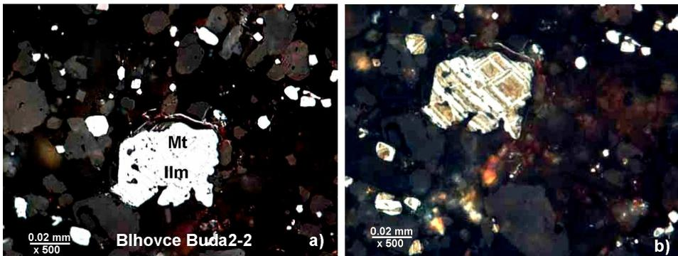
Fig. 5. Olivine basalt Blhovce-Buda; **a)** (in picture) – light microscopy of Fe-Ti grains of the sample; **b)** (in picture) – light microscopy of Bittern-Pattern technique domain structure of Fe-Ti grains of the sample.
