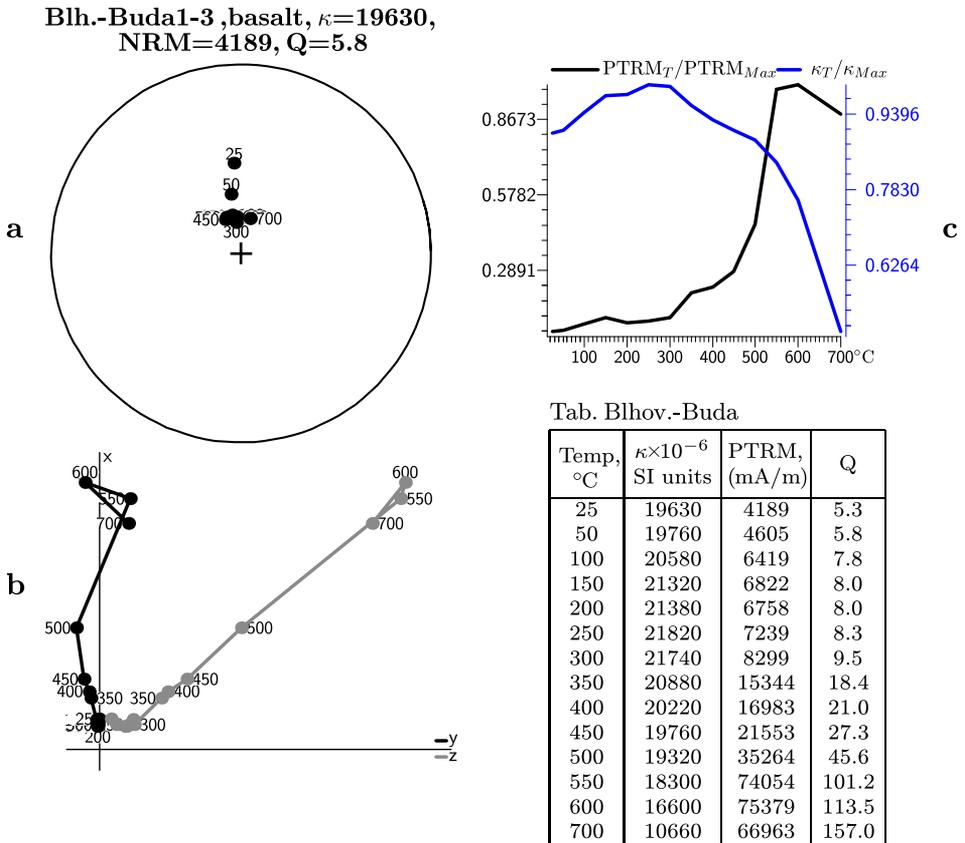
Fig. 4. Stereographic projection, Zijderveld diagram and temperature dependence of PTRM and  $\kappa$ , olivine basalt (magnetic minerals of *pseudo-original phase state*), Blhovce Buda locality, coordinates 48.266° N, 19.957° E. For further description and explanation see Fig. 1.
