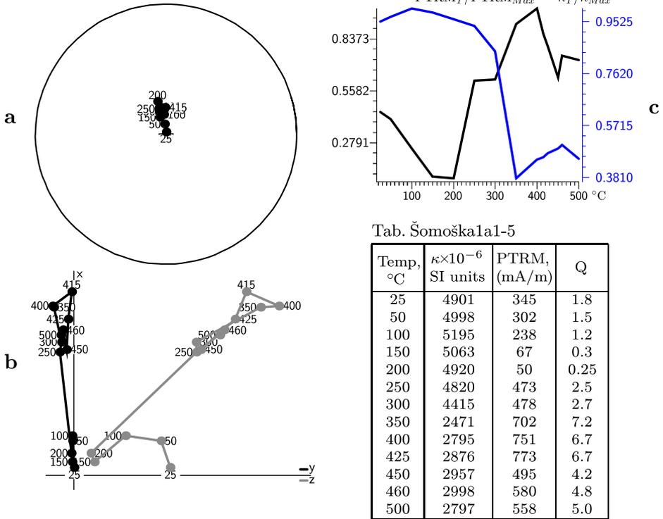
Fig. 13. Thermal magnetization of artificially prepared sample Šomoška-1a1-5G (magnetic minerals of the *pseudo- original phase state*), from olivine basalt lava neck of the Šomoška locality, coordinates (see in Fig. 10); stereographic projection, Zijderveld diagram and temperature dependence of PTRM and  $\kappa$  of sample. G (in the picture) means in gypsum fixed magnetic grains. For further description and explanation see Fig. 1.
