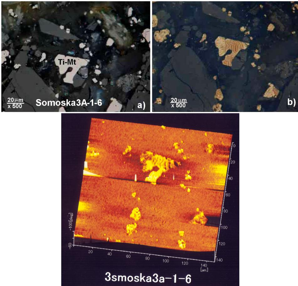
Fig. 15. Olivine basalt Šomoška3a-1-6; **a)** (in picture) – light microscopy of Fe-Ti grains of the sample; **b)** (in picture) – light microscopy of domain structure of Fe-Ti grains of the sample. Picture on bottom: the magneto force microscopy (MFM) image of domain structure of Fe-Ti grains of the sample of the Šomoška locality.
