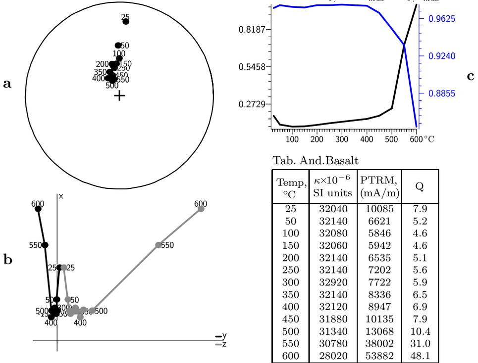
Fig. 6. Stereographic projection, Zijderveld diagram and temperature dependence of PTRM and  $\kappa$ , andesite basalt (magnetic minerals of *pseudo-original phase state*), Malužiná area, coordinates 48.983° N, 19.783° E, age 270 m.y.. For further description and explanation see Fig. 1.
