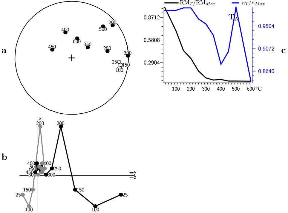
Fig. 8. Thermal demagnetization of the sample B2-11-3 (magnetic minerals of the *transformed phase state*), from nepheline basanite lava flow of the Putikov vršok, coordinates 48.410° N; 18.650° E; stereographic projection, Zijderveld diagram and temperature dependence of PTRM and  $\kappa$  of sample. For further description and explanation see Fig. 1.
