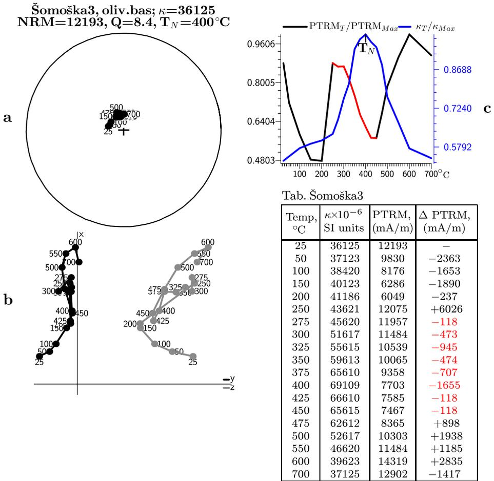
Fig. 11. Thermal magnetization of sample Šomoška3 (magnetic minerals of the *transformed phase state*), from olivine basalt lava dyke of the Šomoška locality, coordinates (see in Fig. 10); stereographic projection, Zijderveld diagram; temperature dependence of PTRM and  $\kappa$  of sample. For further description and explanation see Figs. 1 and 7.
