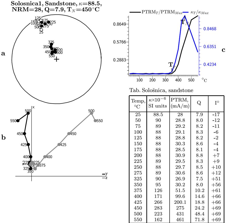
Fig. 19. Stereographic projection, Zijderveld diagram and temperature dependence of PTRM and  $\kappa$ , sandstone, (magnetic minerals of *transformed phase state*), locality Sološnica, coordinates  $48.4654^\circ\text{N}$ ,  $17.231^\circ\text{E}$ , Egemburgian age (24 m.y).  $I^\circ$  – inclination of PTRM of sample. For further description and explanation see Fig. 1.
